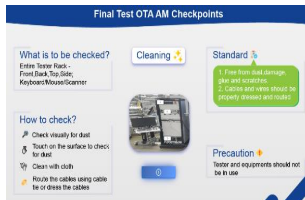
Fig. 3.8: Final Test OTA AM Checkpoints for Entire Cleaning Process
