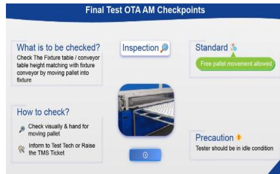
Fig. 3.9: Final Test OTA AM Checkpoints for Entire Inspection Process
