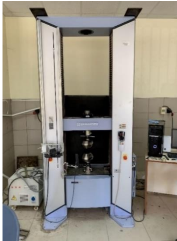
Fig. 2: Universal Testing Machine with a force capacity of 100 KN (SHIMADZU).
