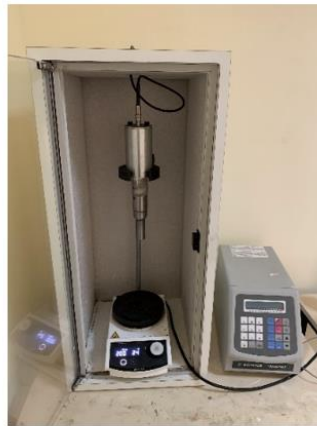
Fig. 3: Ultrasonic processes for small and medium volume application.
