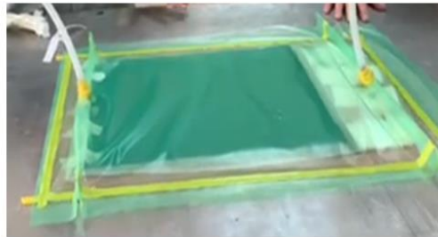
Fig. 2 : Vacuum bag and curing method
