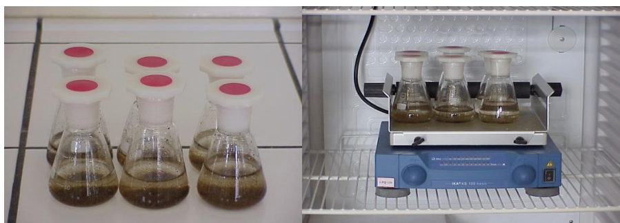
Figure 3: Set of flasks containing metal ions ( \text{Cd}^{2+} , \text{Pb}^{2+} ) and biosorbent
