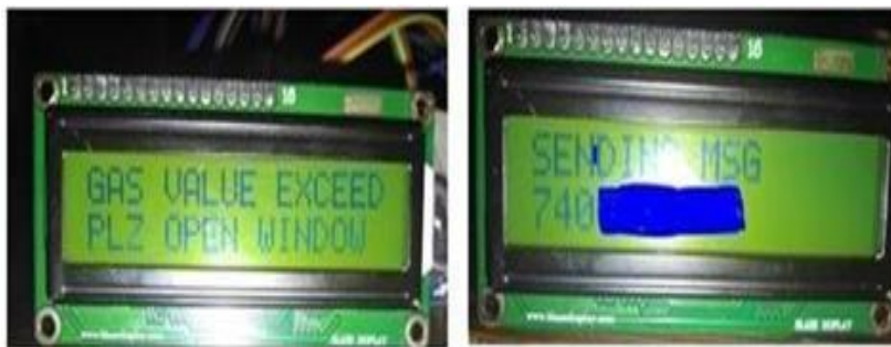
Fig 4. The message got on the predefined proprietor's Mobile Number
