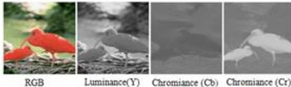
Figure 3: Y, Cb, and Cr components of an RGB image
