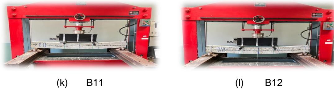
Figure 13: Failure Mode of two-layer Reinforced Concrete Beams
