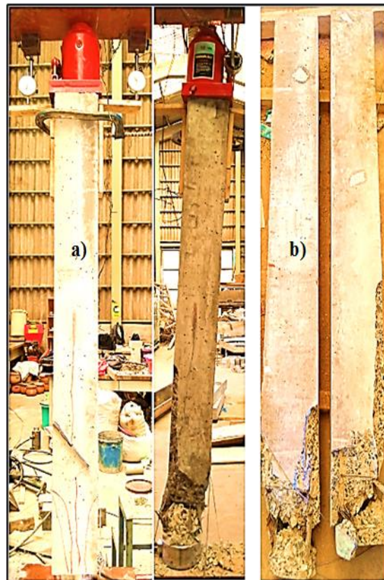
Fig. 7. Failure mode of the BAMT specimens: a) Crack pattern; b) Failure
