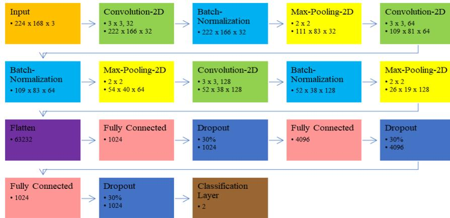
**Figure 3: Proposed CNN architecture for Left and Right Eye Identification in Fundus Images**
