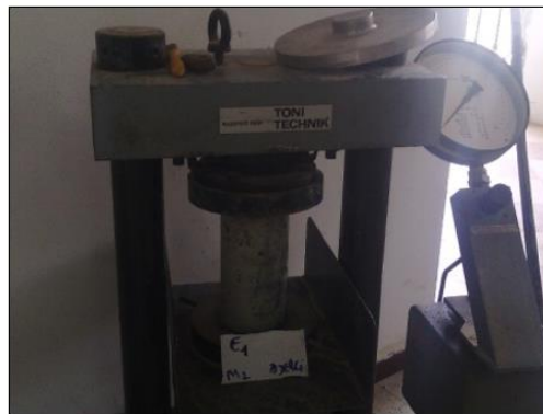
Figure 2: Tony Technik compression machine
