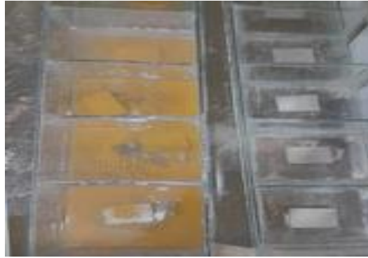
Figure 4: Red sedimentation on the pipe samples
