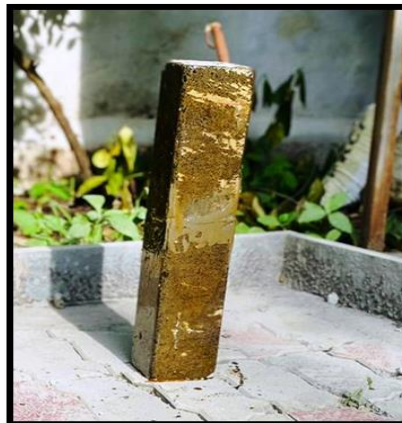
Figure 4: Application of Primer
