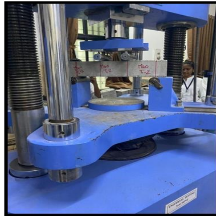
Figure 2: Flexural Test on CFRP Wrapped Specimen
