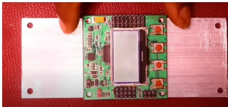
Figure 7: KK2.1.5 flight controller
