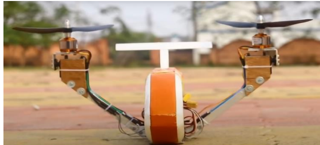
Figure 5: Bicopter Aluminium Frame
