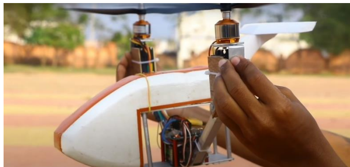
Figure 6: Bicopter Tilting Mechanism
