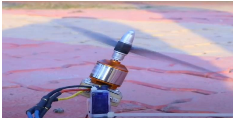
Figure 8: Tricopter rear motor with tilt function
